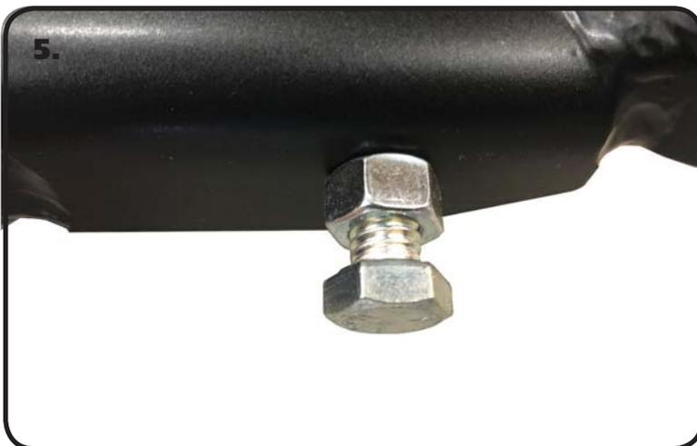
5. Thread the 3/8"-16 nut onto the 3/8"-16 x 1 1/4" bolt. Thread it into the front hole of the ball joint plate. You will need to adjust the steering stop to suite your needs. This setting will vary depending on wheel and tire size and other suspension components.
