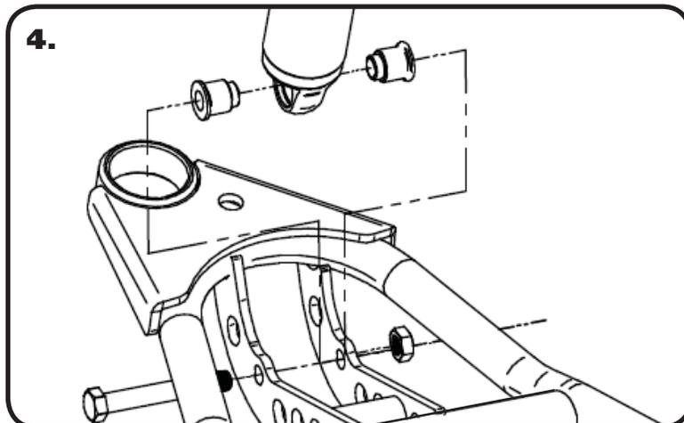
4. Insert the Bearing Spacers into the lower shock bearing. The SMALL end goes into the bearing. Swing the Control Arm up, line up the 1/2" holes with the bearing spacers, insert 1/2"-20 x 3 1/2" bolt. Install a 1/2" flat washer and nylok nut.
