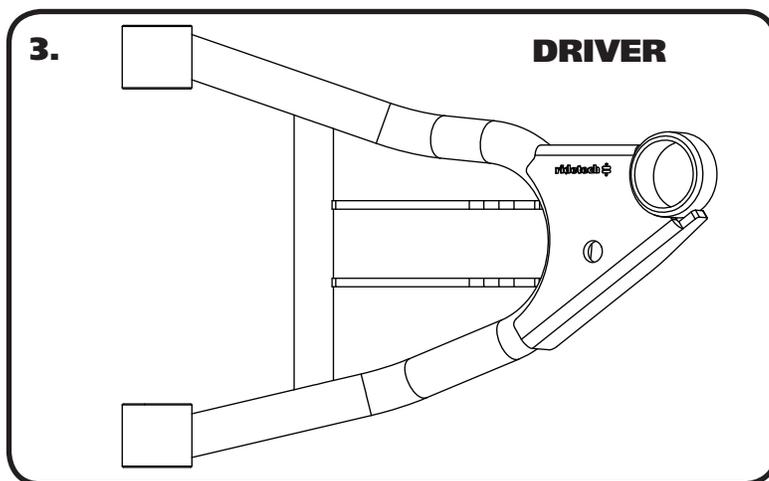
3. After removing the factory lower control arm, clean the bushing mounting surfaces on the frame. The Control Arms are marked "D" for Driver and "P" for Passenger. The Balljoint Pin points up and the Sway bar mount is on the front side of the arm. Fasten the lower arm to the frame with the hardware supplied. Note: On some cars the frame brackets may be pinched and will need to be spread back apart to allow the bushing to slide in.
