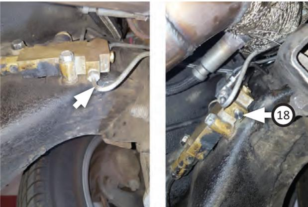
8. Remove right front brake line from bottom of proportion valve and install **inverted flare plug fitting (18)**.
