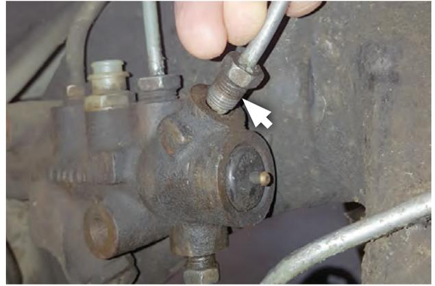
10. Remove left front brake line from top of proportion valve.
