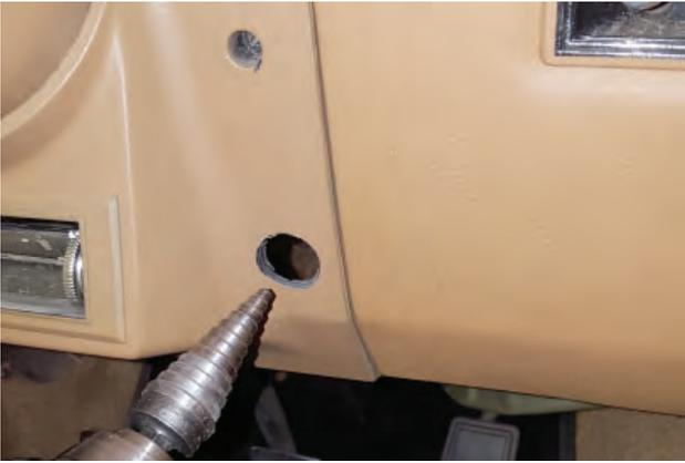
16. As long as your layout follows wiring diagram (page 5), there are many ways to mount **on/off switch (9)** and **momentary button (8)**, keyed power preferred. The pictures on this page show a mounting layout that worked well for this application.
