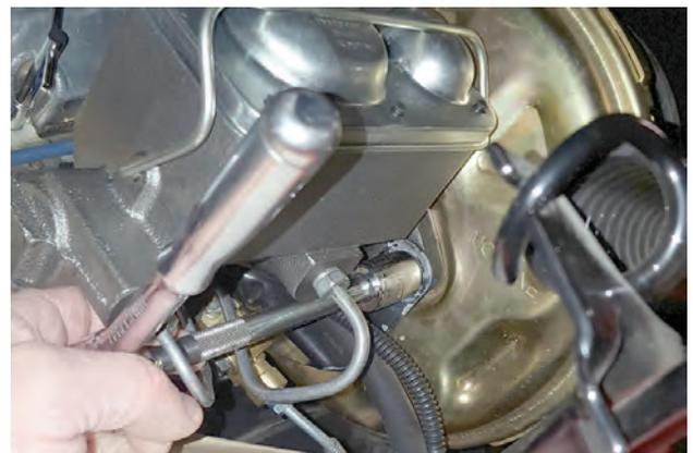
6. Remove (x2) nuts that mount master cylinder to brake booster. Do NOT remove master cylinder.
