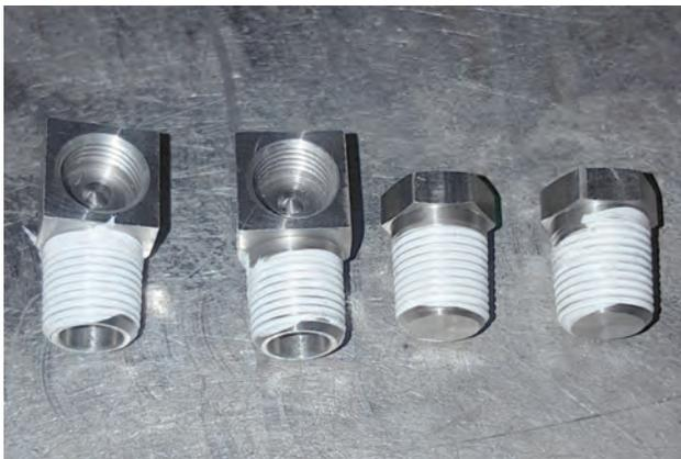
2. Apply teflon tape to all pipe thread fittings.
