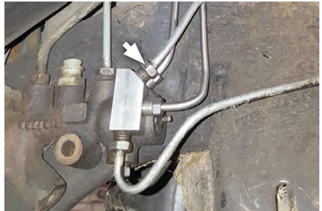
11. Insert left front brake line into top of inverted flare fitting.
