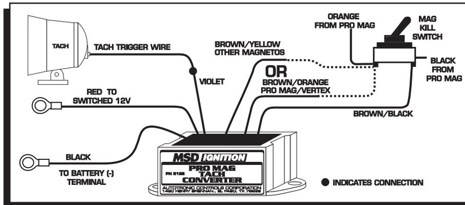
Figure 3 Wiring a Tachometer with PN 8132.
