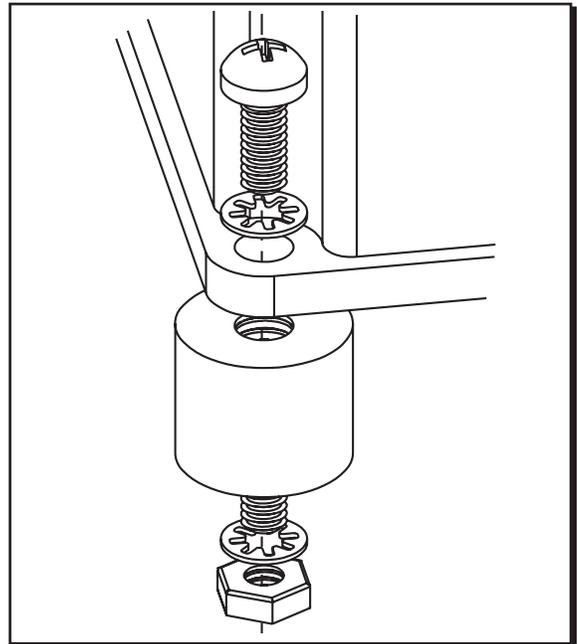
**Figure 1 Mounting the Points Box.**
