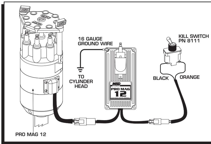
Figure 2 Wiring the 12 Amp Pro Mag.
