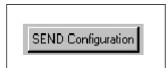
When finished sending the message “**Device Programmed Successfully**” should be displayed at the bottom of the progress box. If you receive an error message, turn power to the system off and then back on and repeat the send configuration process. If problems persist, check the troubleshooting section in your manual and then contact RacePak. Save your configuration file to disk and update the Module Configuration Setup Box on the front of this worksheet with the new setup configuration.
