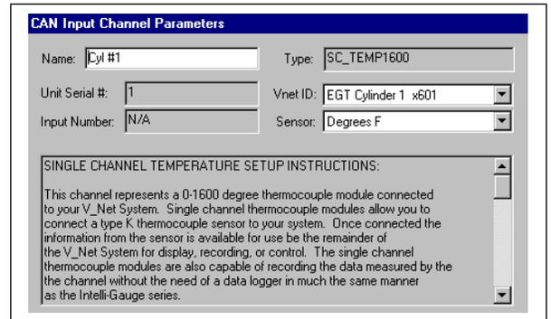
Locate the text box labeled **Single Channel Temperature Setup Instructions**. This text box provides online instructions for modifying the setup of this module. Read the instructions and modify the setup as desired. (Please note the scroll bars located on the left- hand portion of the text box is used to scroll through the instructions).
